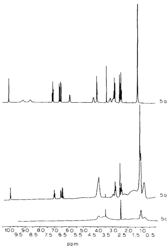
Fig. 5.  $^1\text{H-NMR}$  spectra corresponding to: (a) carteolol hydrochloride, (b) Eudragit L-carteolol complex, (c) Eudragit L-Na 30%.
