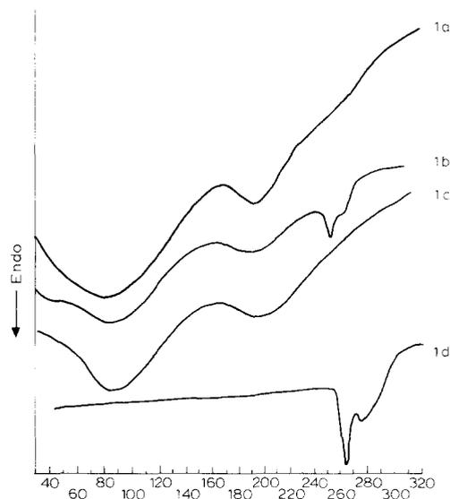
Fig. 1. Thermograms corresponding to: (a) Eudragit L-Na 30%, (b) physical mixture Eudragit L-Na: carteolol (1:1), (c) Eudragit L-carteolol complex, (d) carteolol hydrochloride. Abscissa: temperature (°C).
