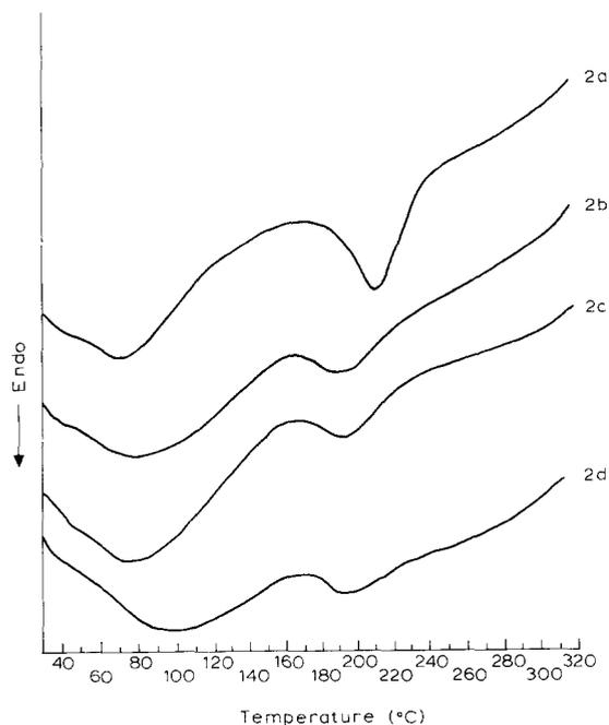
Fig. 2. Thermograms corresponding to: (a) Eudragit® L 30D, (b) Eudragit L-Na 30%, (c) Eudragit L-Na 35%, (d) Eudragit L-Na 40%.
